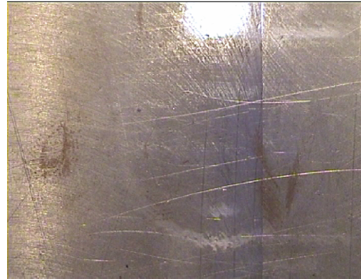
Liner wall with intact lubrication film
